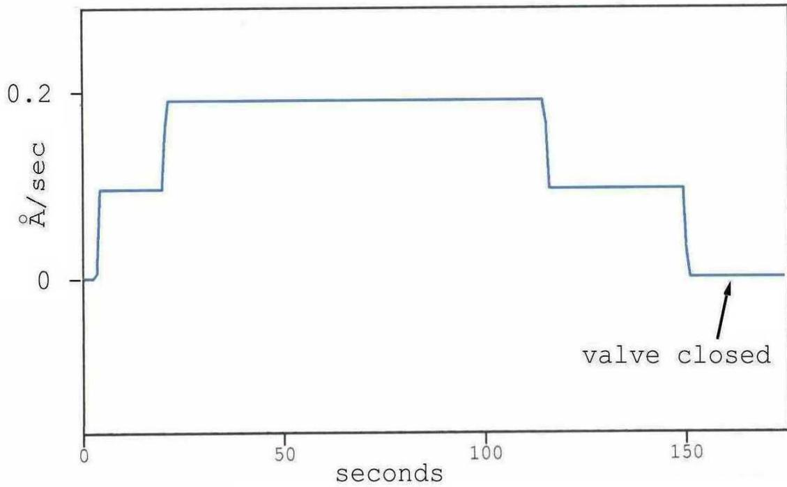
Figure 2b: Deposition of atomic antimony vapour as a function of valve position.
