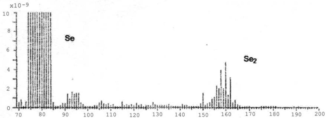
Figure 4a: A mass spectrum of species from a pure Selenium discharge.
