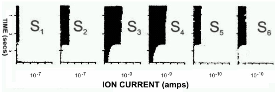
Figure 4b: A mass spectrum of a 40W discharge in pure sulphur, showing the dominance of the monomer and dimer
