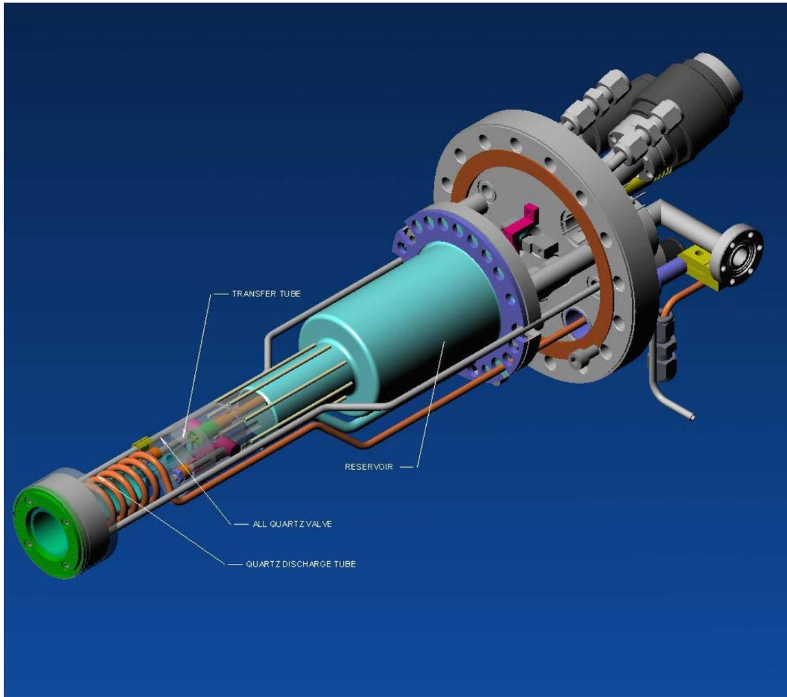
Figure 1: Illustration of all-quartz valved RF cracker
