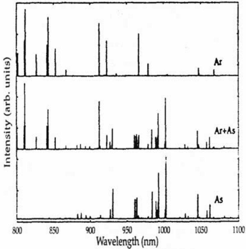
Figure3: Emission spectrum of argon-supported and pure As discharges
